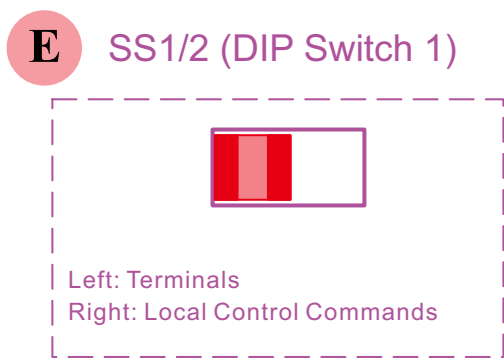
Figure 8 SS1/2 Position in Terminal Control Mode
